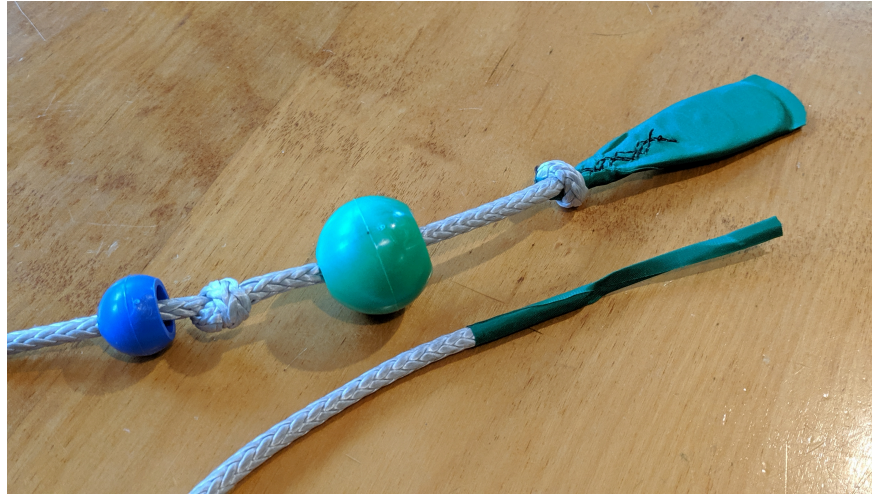
Figure 2.3: Grip end of the trim line with balls offset to show knots (above) and thread end (below)
