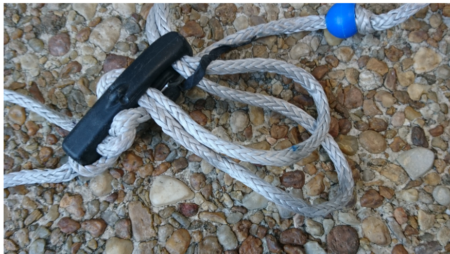
Figure 3.4: Take the slack out of the trimline loops 2 of 3.
