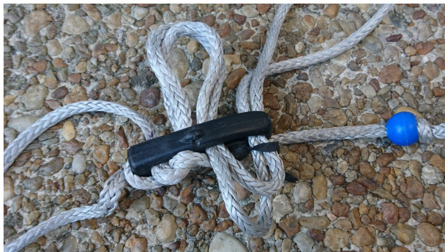
Figure 3.3: Route the insignia cloth tail through the loops. Holding the tail in place, pull the trim line slack down through the cleat grooming the lines as you go. Keep the lines as parallel as possible. Take the slack out of the trimline loops 1 of 3.
