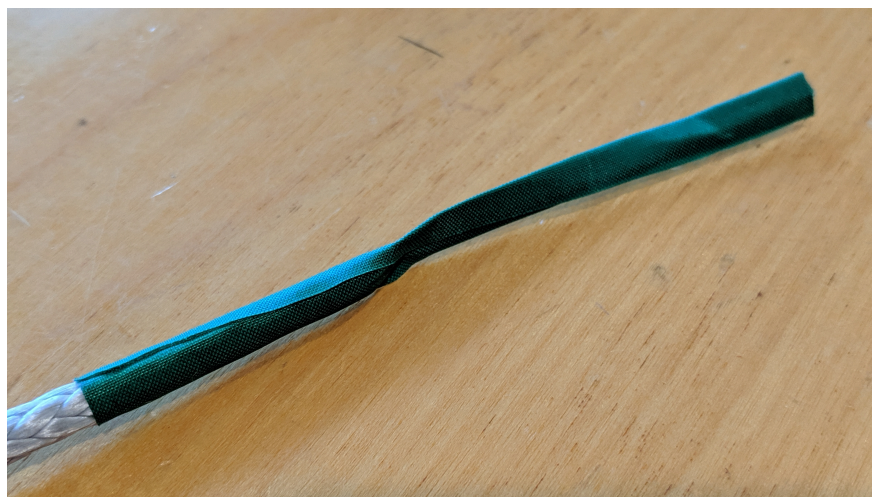
Figure 2.2: Threading end of the trim line formed with a wrap of insignia cloth
