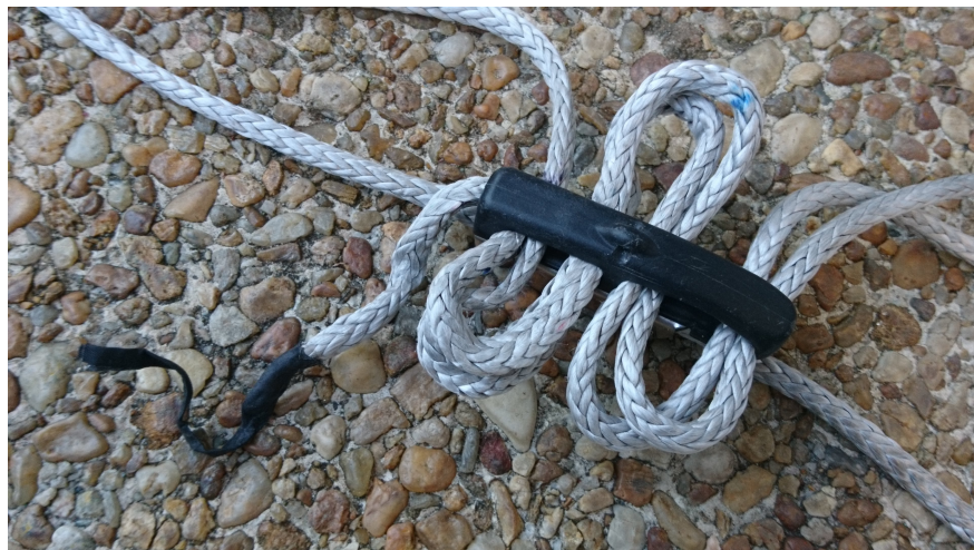
Figure 3.1: Form large parallel loops of line on each side of the cleat's serpentine path. Route about 5cm of the trim out of the top of the cleat.
