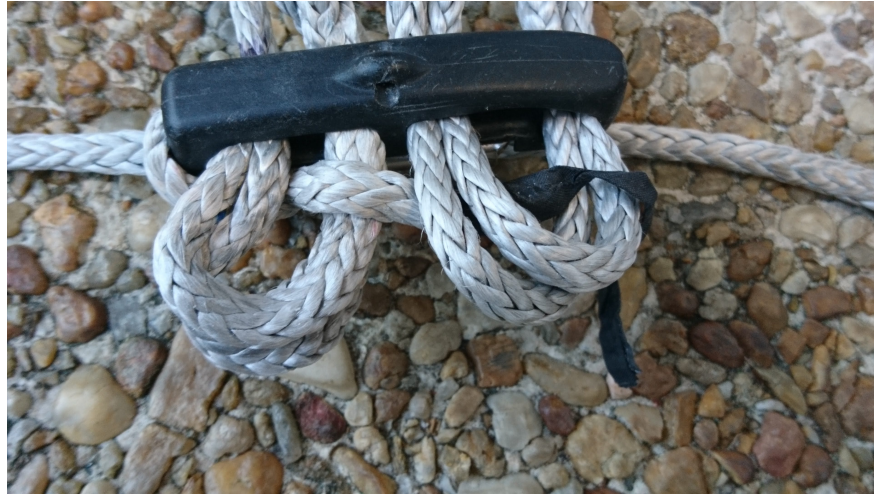
Figure 3.2: Route the 5cm of trim line tail through the loops along the side of the serpentine.
