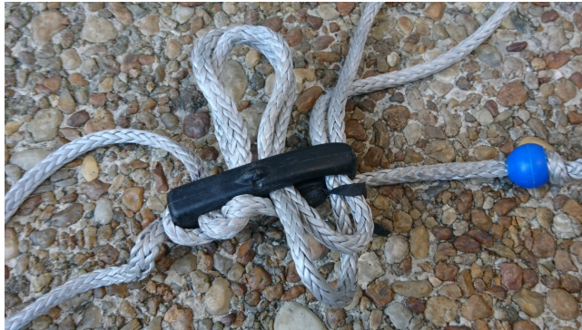
Figure 3.4: Route the insignia cloth tail through the loops. Holding the tail in place, pull the trim line slack down through the cleat grooming the lines as you go. Keep the lines as parallel as possible. Take the slack out of the trimline loops 1 of 3.
