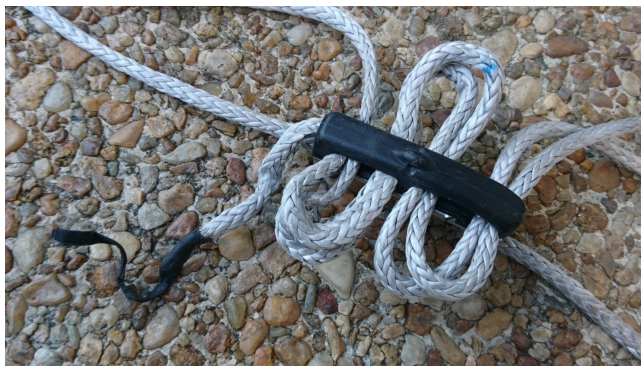
Figure 3.2: Form large parallel loops of line on each side of the cleat's serpentine path. Route about 5cm of the trim out of the top of the cleat.
