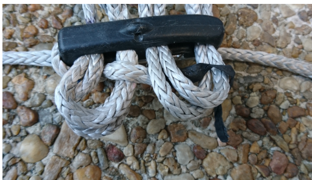
Figure 3.3: Route the 5cm of trim line tail through the loops along the side of the serpentine.
