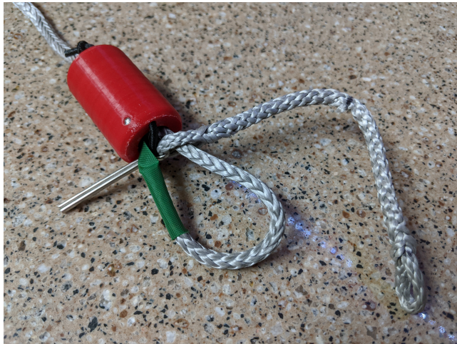
Figure 3.1: Threading the trim line through the Mini-chickenloop
