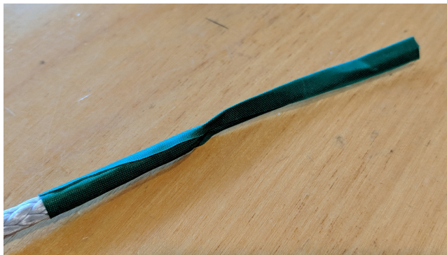
Figure 2.3: Threading end of the trim line formed with a wrap of insignia cloth
