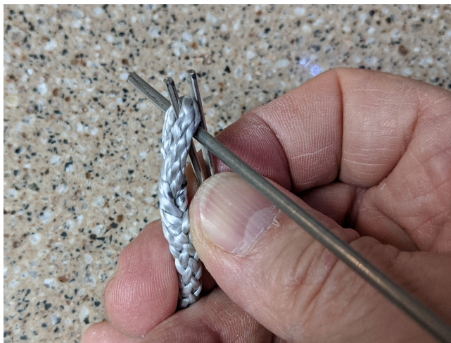
Figure 2.16: Installing the cotter pin on the chickenloop line
